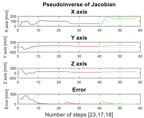
Fig. 4. Simulation result of DOBOT axes and total error of coordinates.
