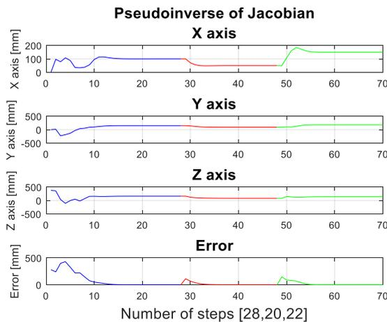
Fig. 3. Simulation result of DOBOT axes and total error of coordinates.
