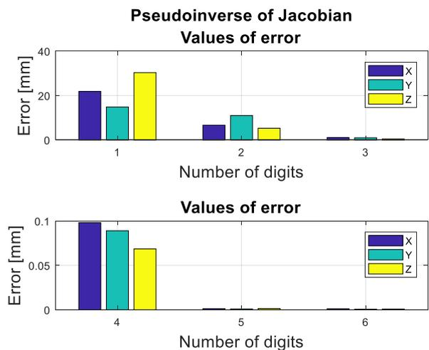
Fig. 5. Simulation result of total error of coordinates from 1 to 6 digit.
