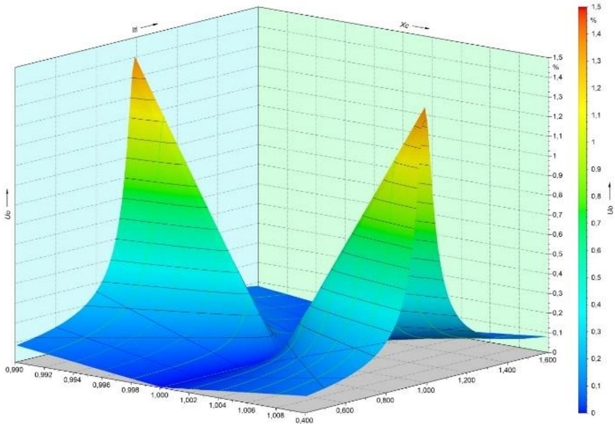
Fig. 2. Graph showing the impact of cross parameters  $X_C$  unbalance (ideally, a balanced network equals  $X_C = 1$ ) and the impact of the arc-suppression coil tuning accuracy  $I_{q1}$  (in a resonant state  $I_{q1} = 1$ ) on the zero sequence voltage  $U_0$ .
