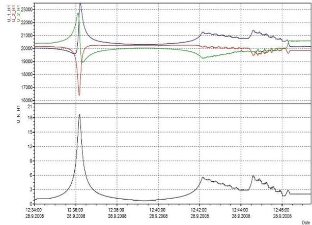
Fig.5. Tuning of an arc-suppression coil in an asymmetrical network with a blocked function of automatic voltage symmetrization (on the left) and with the unblocked function (on the right).
