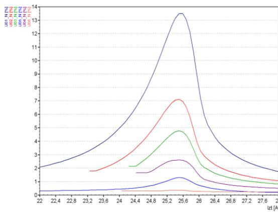
Fig.4. Controlling capacitive asymmetry in a network using the VSS system, changes in the zero sequence voltage during arc-suppression coil tuning.
