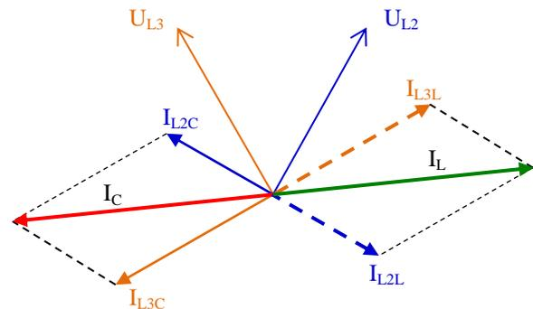
Fig.6. Earth fault current elimination in a network with a major phase-to-ground capacity unbalance with an earth fault in  $L_1$  phase ( $U_{L1} = 0$ ).
