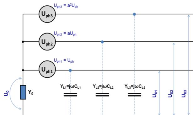
Fig. 1. A simplified diagram for the following calculation of the phase voltage in a network.
