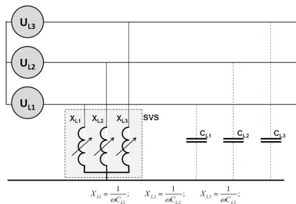
Fig.3. Basic diagram of VSS connection.
