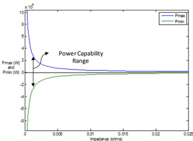
Fig. 10. Power range capability for changing impedance.
