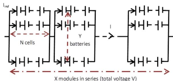
Fig. 8. A simple configuration of a battery pack.
