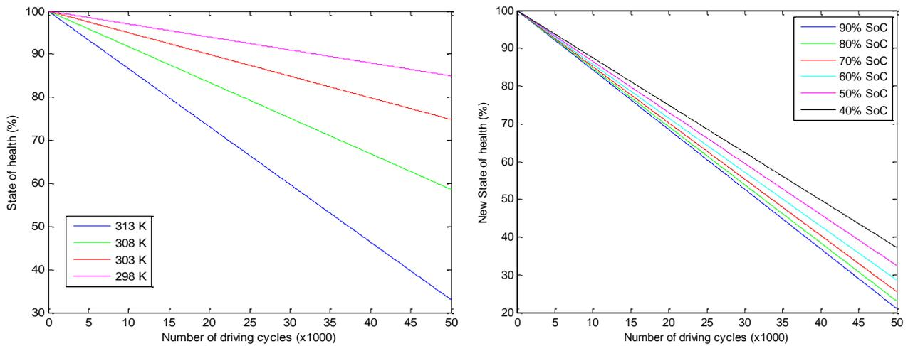
Fig. 4. SoH calculation different initial SoC and temperature.
