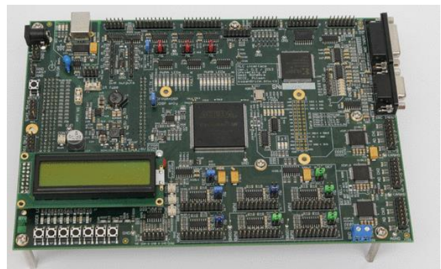
Fig. 7. MLC interface – control system with DSP and FPGA.
