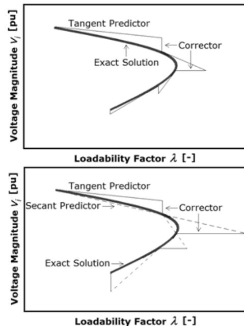
Fig. 1. Predictor/Corrector Mechanism for the CLF Analysis [10].
